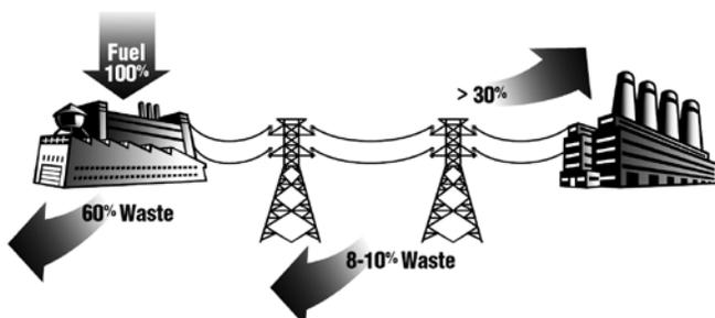
Figure 1 - Today's "grid" system of central power plants and transmission lines wastes much of the energy in the original fuel.
