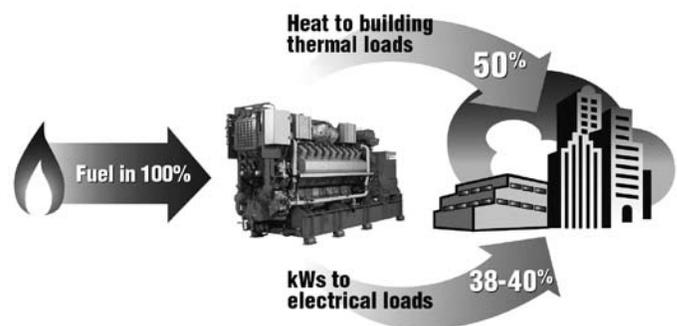
Figure 2 - CHP plants operate at twice the average efficiency of the U.S. power system.
